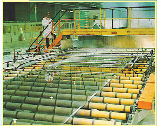
A long, flat layer of cooled glass comes out of the lehr to be washed and cut.
